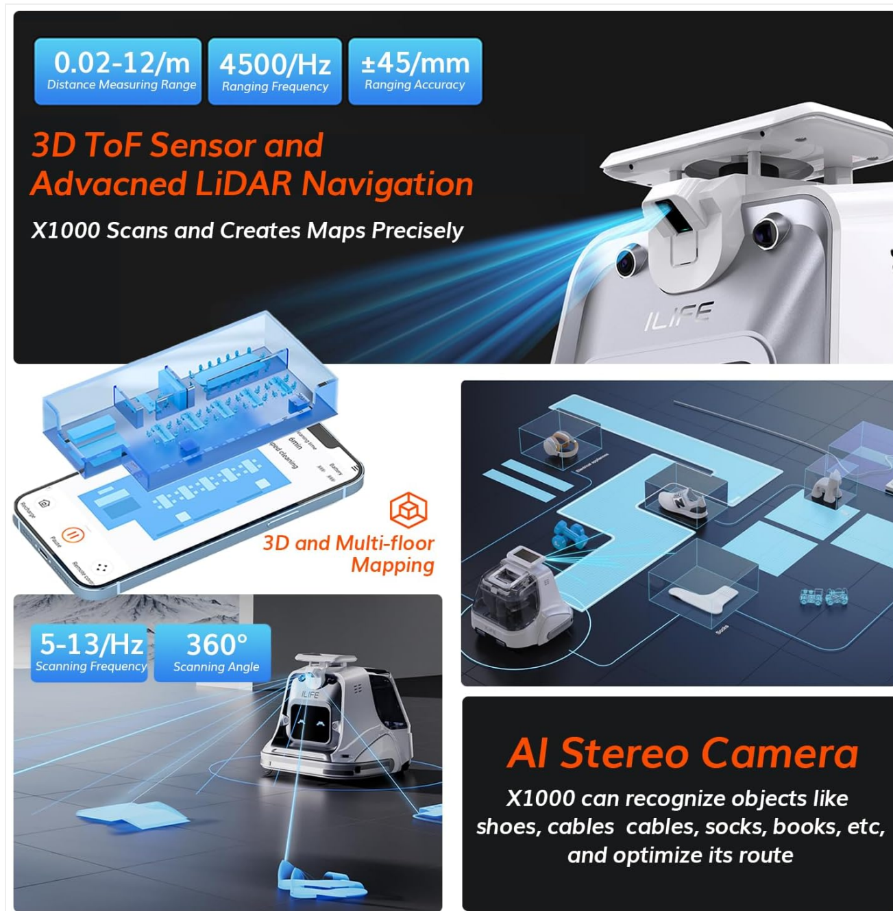
Figure 3.4: Illustration of the robot's advanced navigation system, including 3D ToF sensors, LiDAR technology for precise mapping, and AI stereo camera for object recognition.
