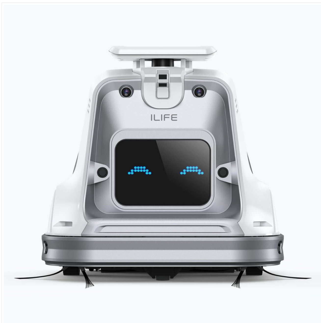
Figure 3.1: Front view of the ILIFE X1000 Robotic Vacuum Cleaner, showing the main body, front bumper, and side brushes.
