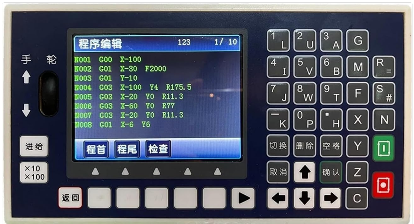
Figure 6.1: Example of a G-code program displayed on the TC55H controller screen.
