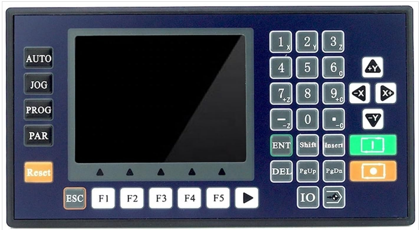
Figure 4.1: The front panel of the HEXEH TC5530V controller, showing the 3.5-inch color LCD screen and the integrated keypad for operation and programming.
