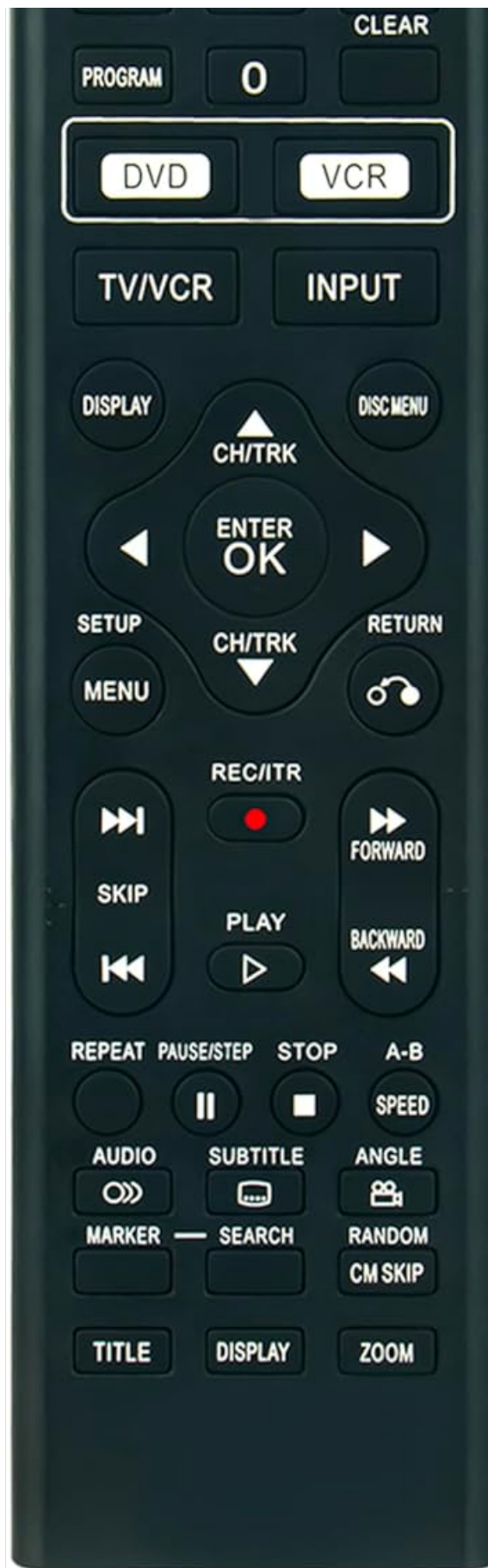
Figure 2.1: Front view of the VINABTY 6711R1P081G remote control. This image displays the layout of all control buttons, including power, numerical keys, DVD/VCR mode selection, navigation, and playback controls.
