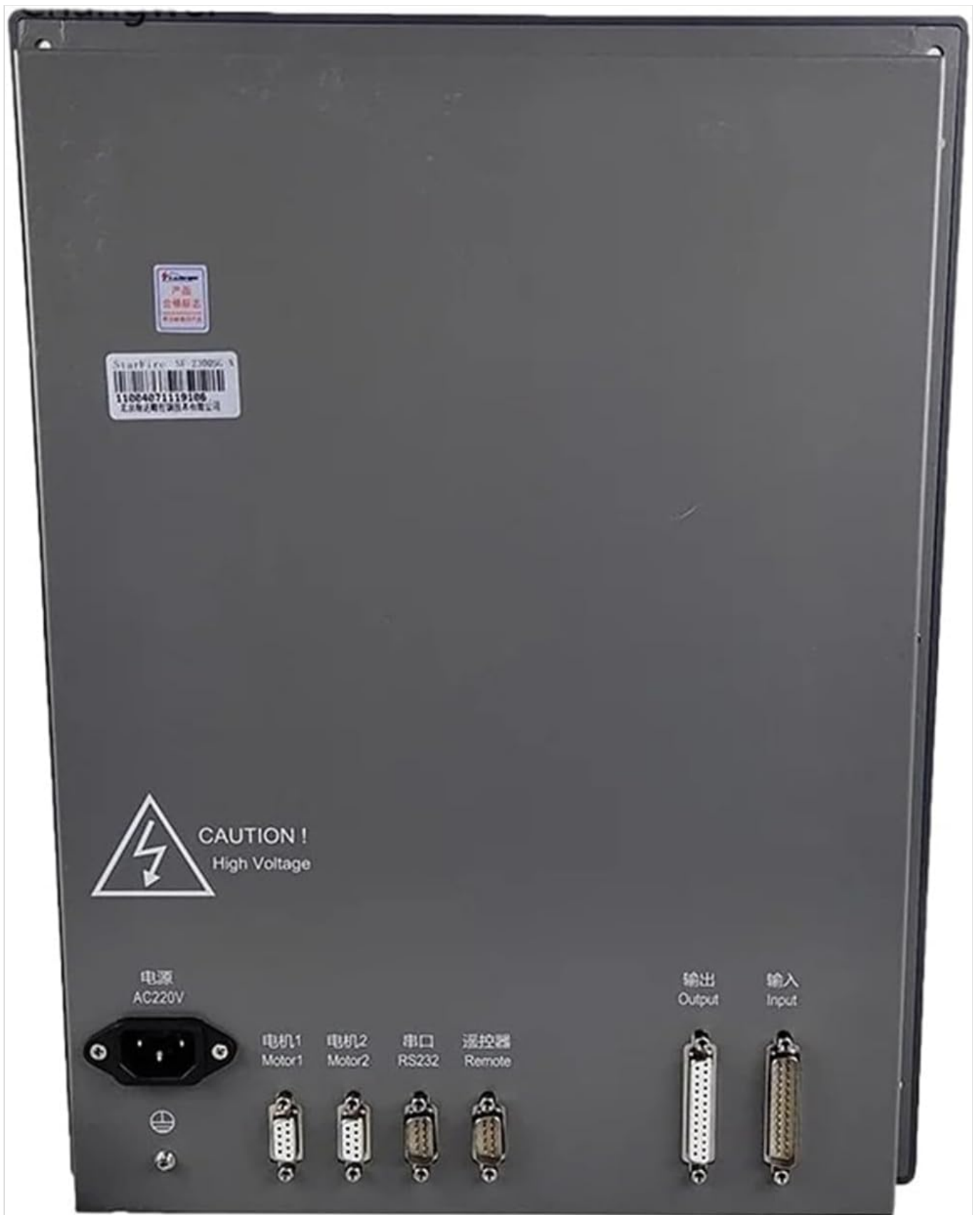
Figure 4.2.1: Rear panel of the HEXEH SF-2300S controller showing various connection ports. From left to right: AC220V power input, Motor1, Motor2, RS232, Remote, Output (14-way), and Input (16-way).
