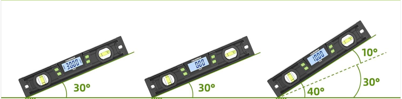
Figure 5.3: Illustration of relative angle measurement. The level is first set to 0° on a 30° surface, then moved to a 40° surface, displaying a relative angle of 10°.
