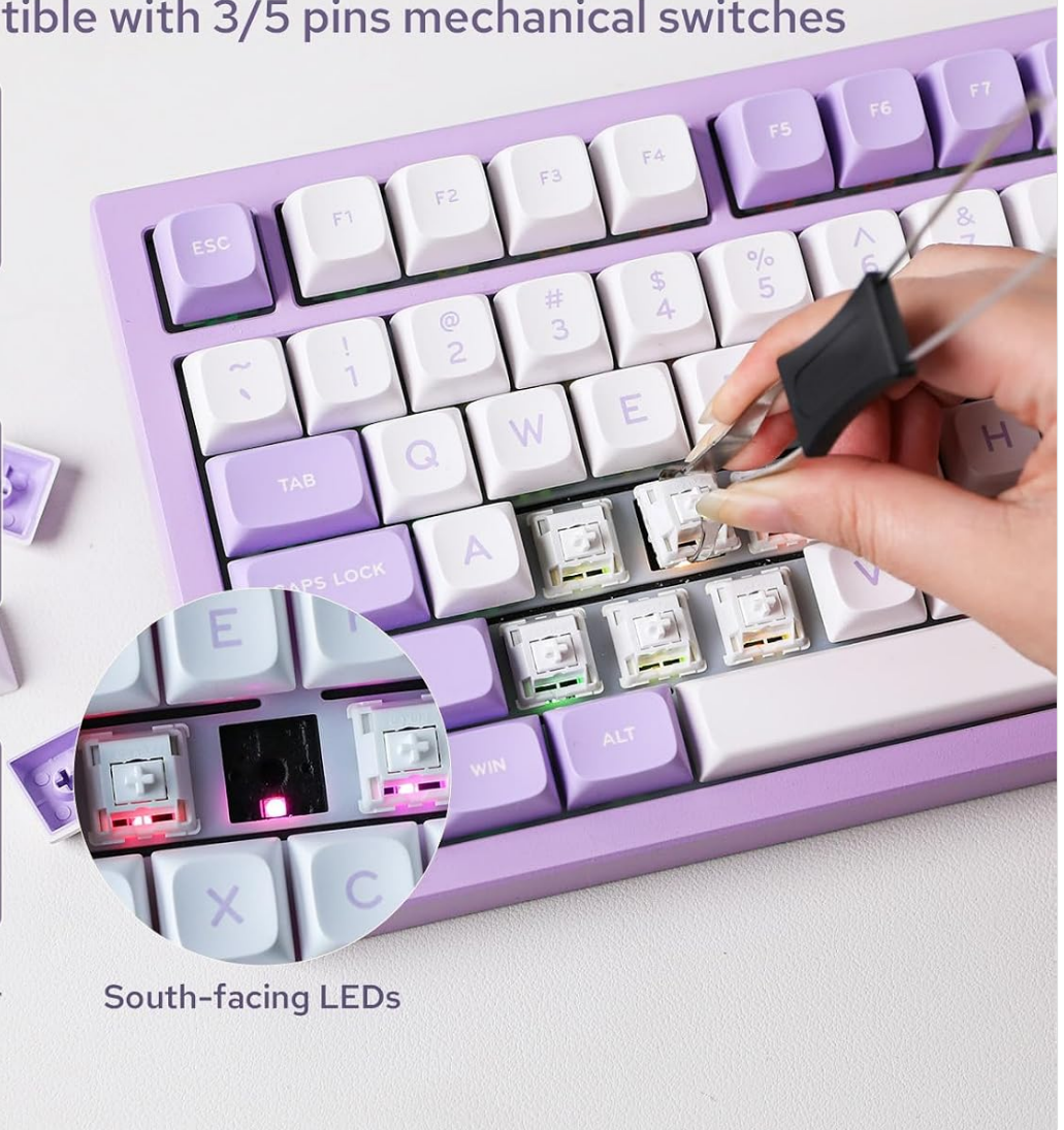
Figure 5: Demonstration of the hot-swappable PCB, compatible with 3/5-pin mechanical switches.
