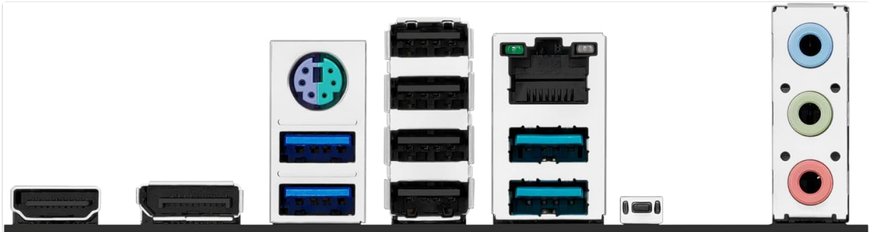
Image 3.2: The rear input/output panel of the motherboard, showing various ports for external devices.
