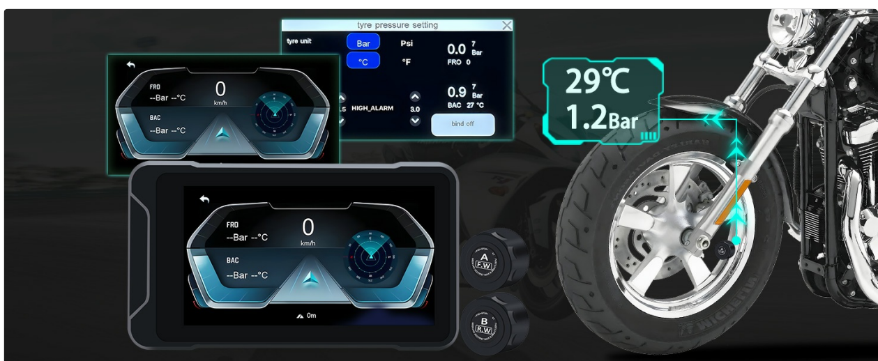
Figure 3.4: TPMS settings interface. This image shows the user interface for the tire pressure monitoring system (TPMS), allowing adjustment of pressure units and alarm thresholds, along with real-time display of tire data.
