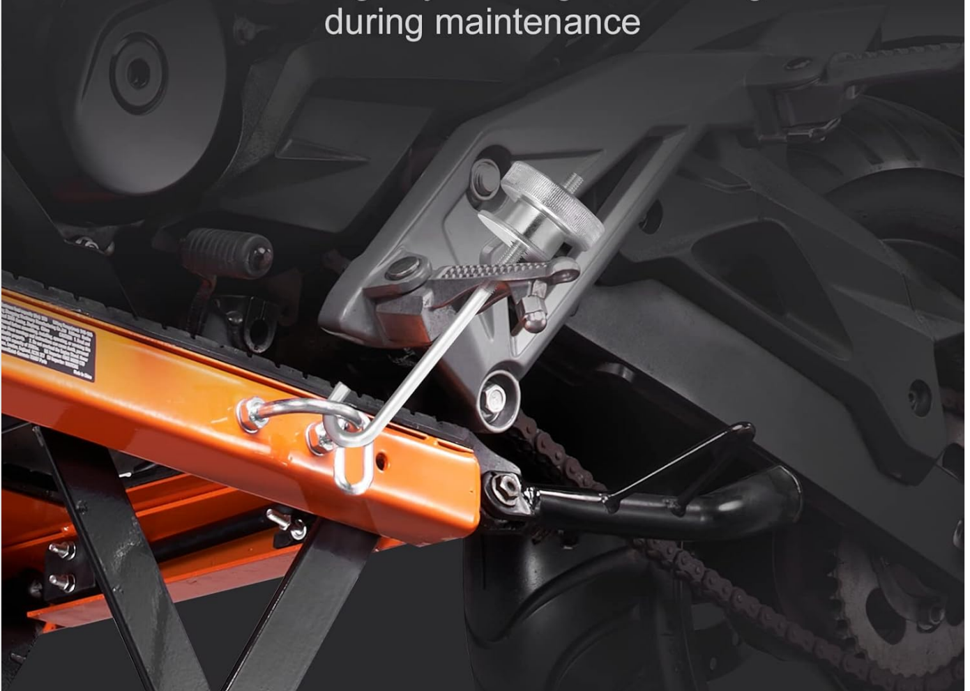
Figure 6: Shows the J-hook attachment point for enhanced stability of the motorcycle on the platform.
