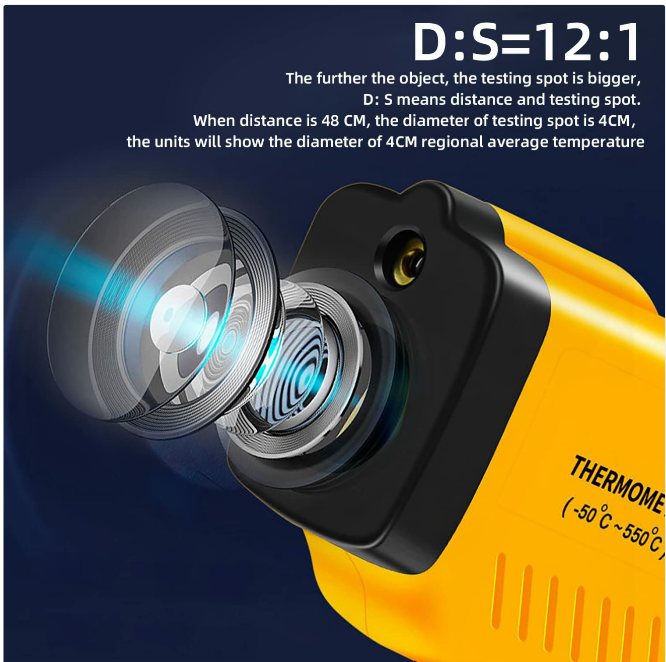
Figure 5.1: Understanding the 12:1 Distance to Spot ratio is crucial for accurate temperature readings, indicating the measurement area relative to distance.
