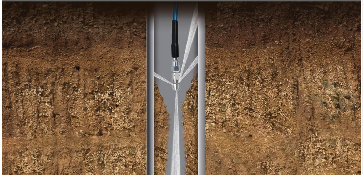
Image: Depiction of the nozzle clearing a clog inside a pipe.
