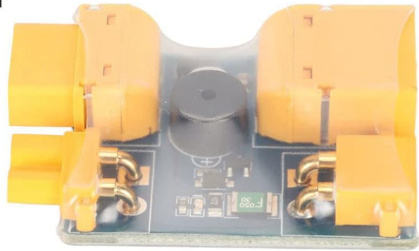
Figure 3.2: Detail of the XT30 and XT60 input/output connectors.
