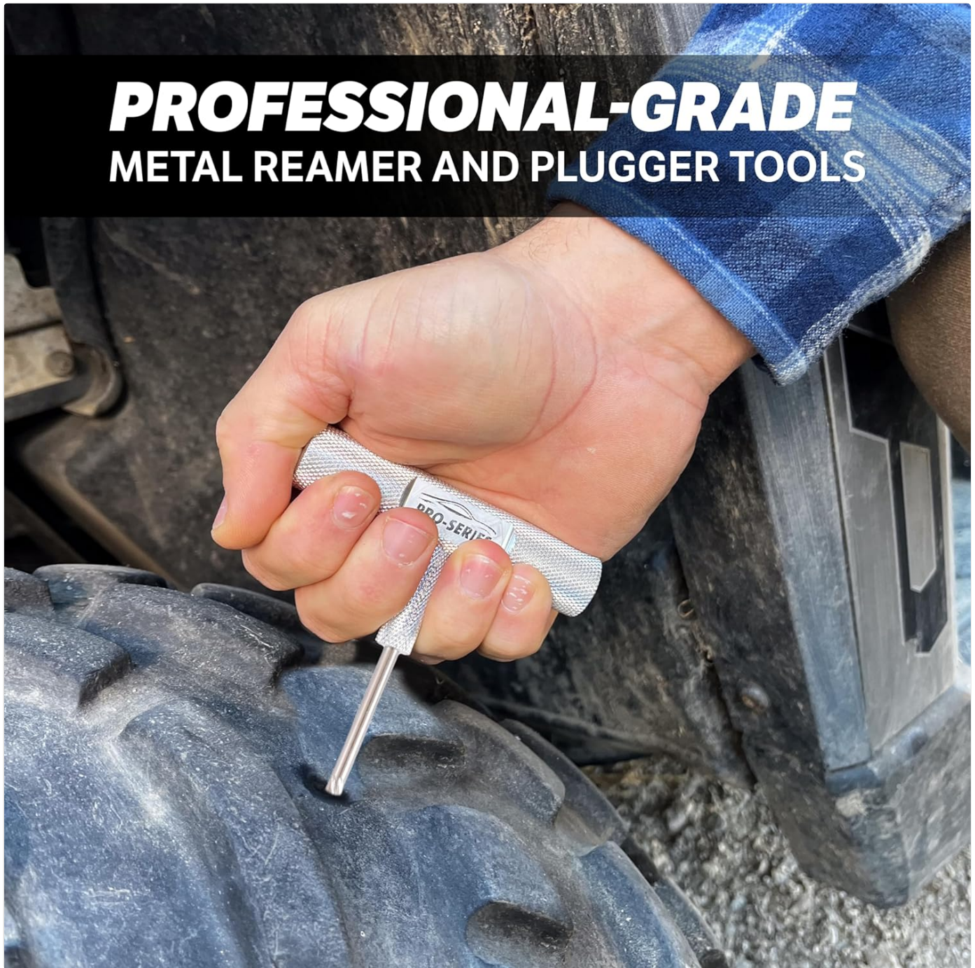
Image: A hand demonstrating the use of the T-handle reamer tool to prepare a tire puncture for repair.
