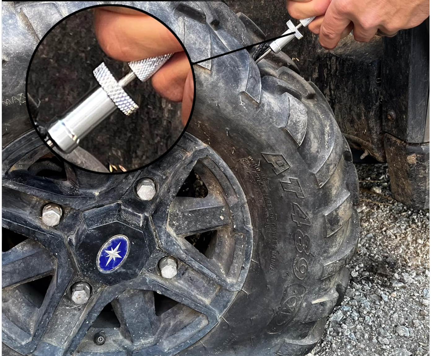
Image: A close-up of a hand inserting a black tire string into the eye of the T-handle plugger tool, ready for insertion into the tire.
