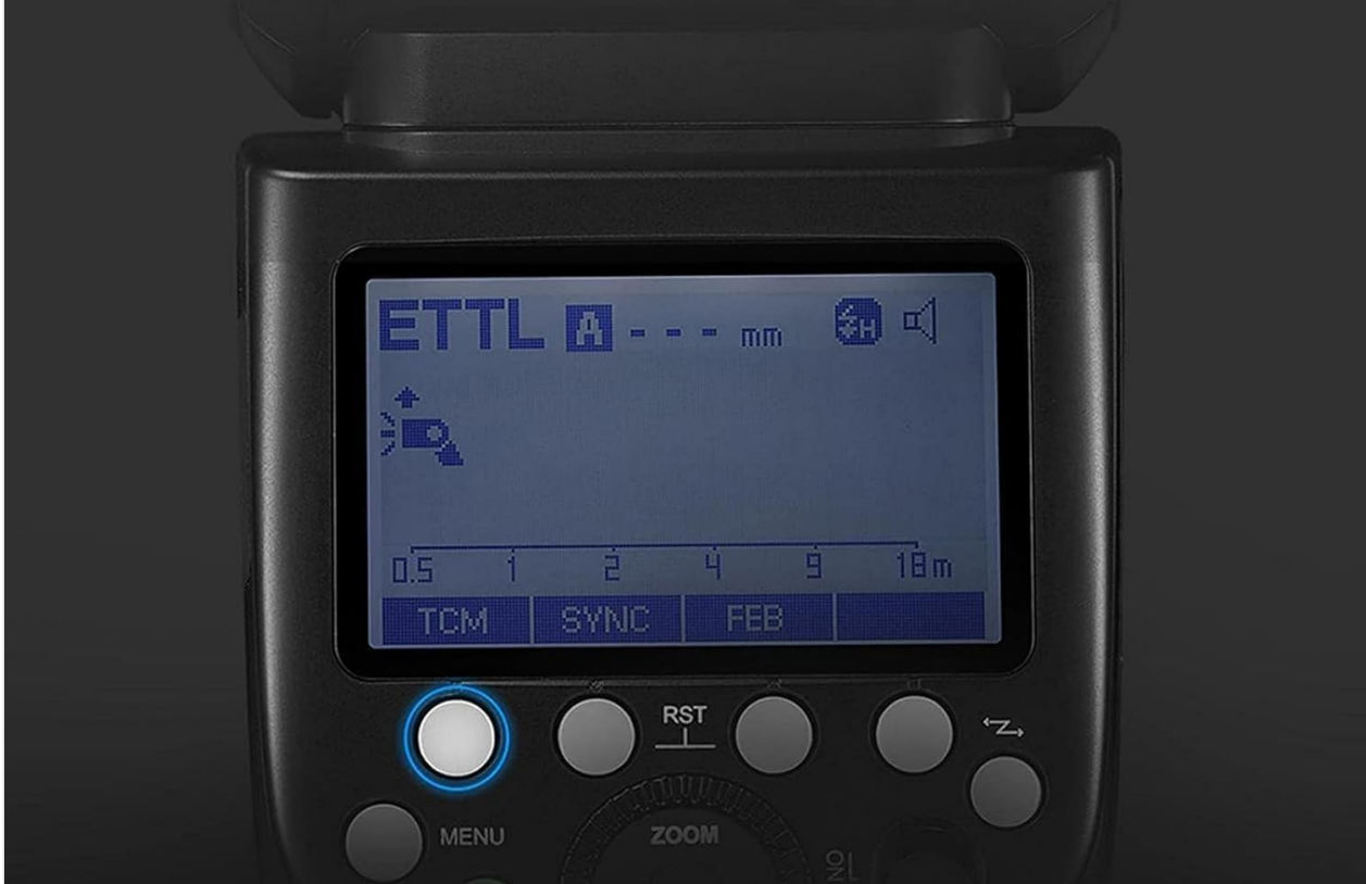
Image: The LCD screen of the Godox TT685IIC displaying the TCM function, indicating the conversion from TTL to manual mode.
