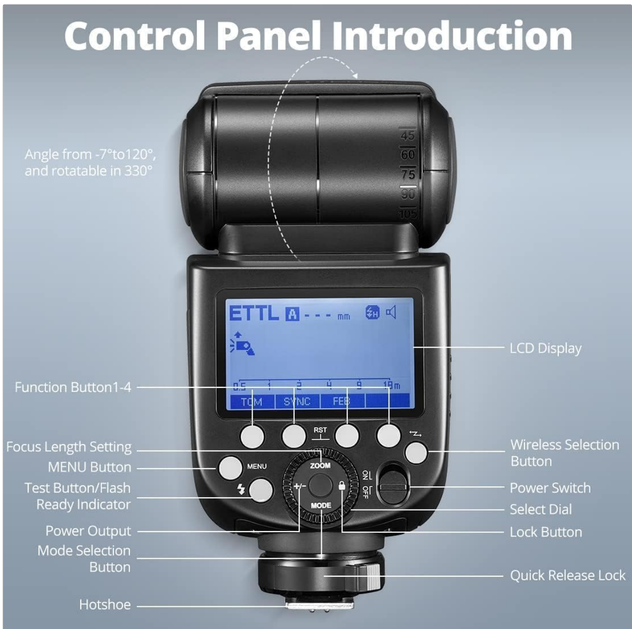
Image: Detailed diagram of the Godox TT685IIC control panel, labeling the LCD display, function buttons, menu button, test button/flash ready indicator, power output, mode selection button, focus length setting, wireless selection button, power switch, lock button, quick release lock, and hotshoe.
