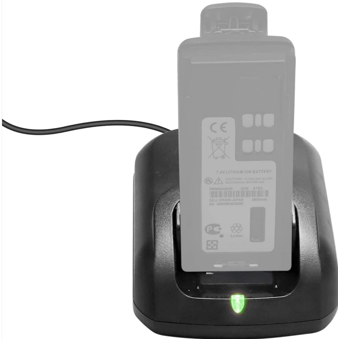
Figure 3.4: A battery correctly placed in the charger, showing the charging indicator light.
