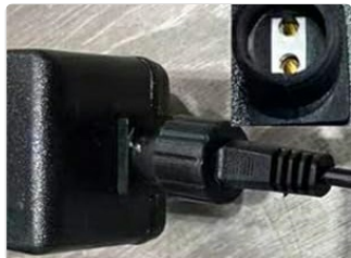
Plug for the LED light component.
