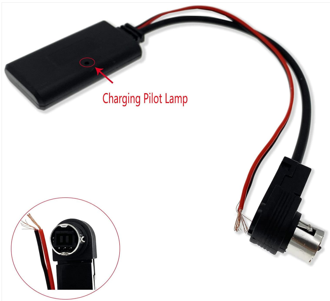
Figure 5.2: The Bluetooth module features a charging pilot lamp, which indicates power status.
