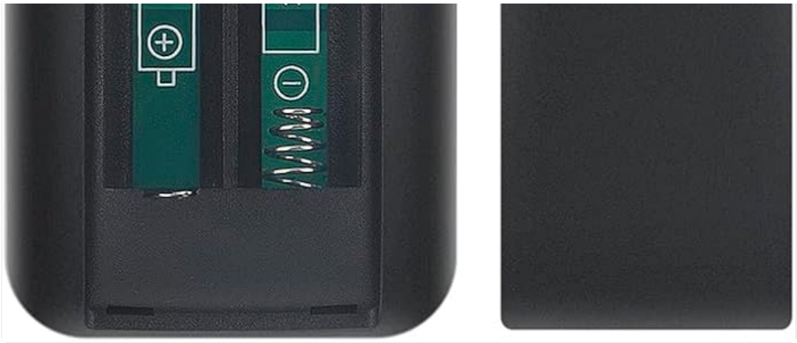
Image 3.1: Back of the remote control with the battery compartment open, illustrating correct battery placement.
