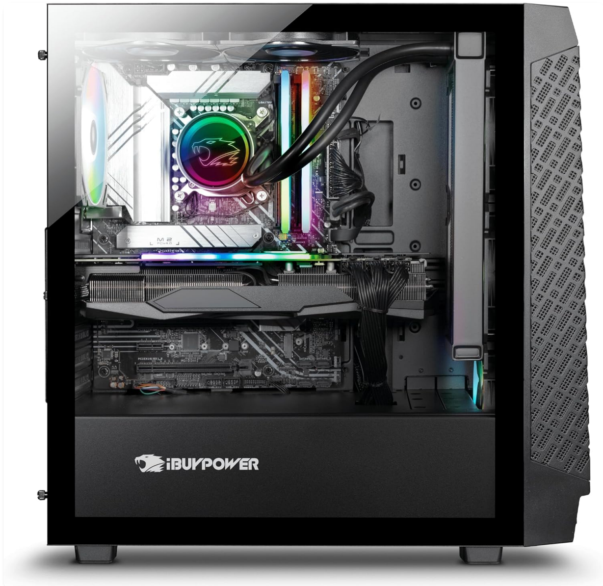
Figure 2: Interior view of the PC, showing the CPU cooler, RAM, and GPU. Ensure all internal packaging is removed.
