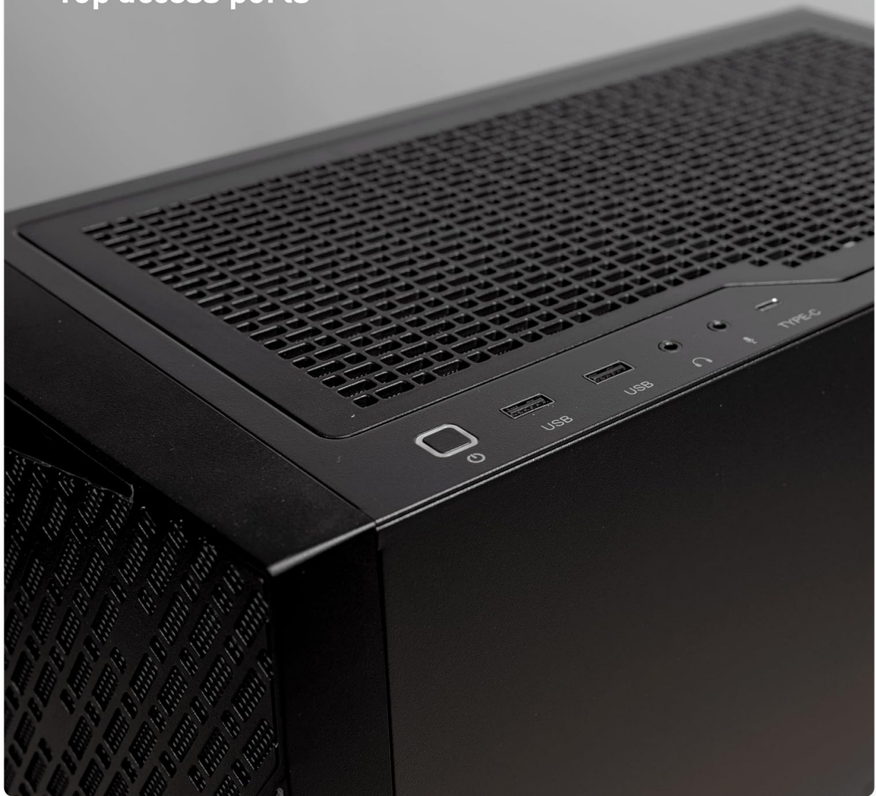
Figure 4: Top access ports for convenient USB and audio connections.
