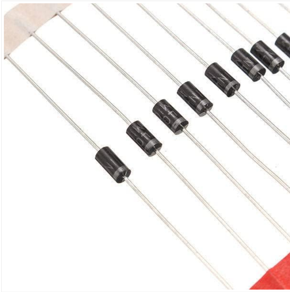
Figure 4.1: Close-up of IN4007 diodes, highlighting the cathode band.
