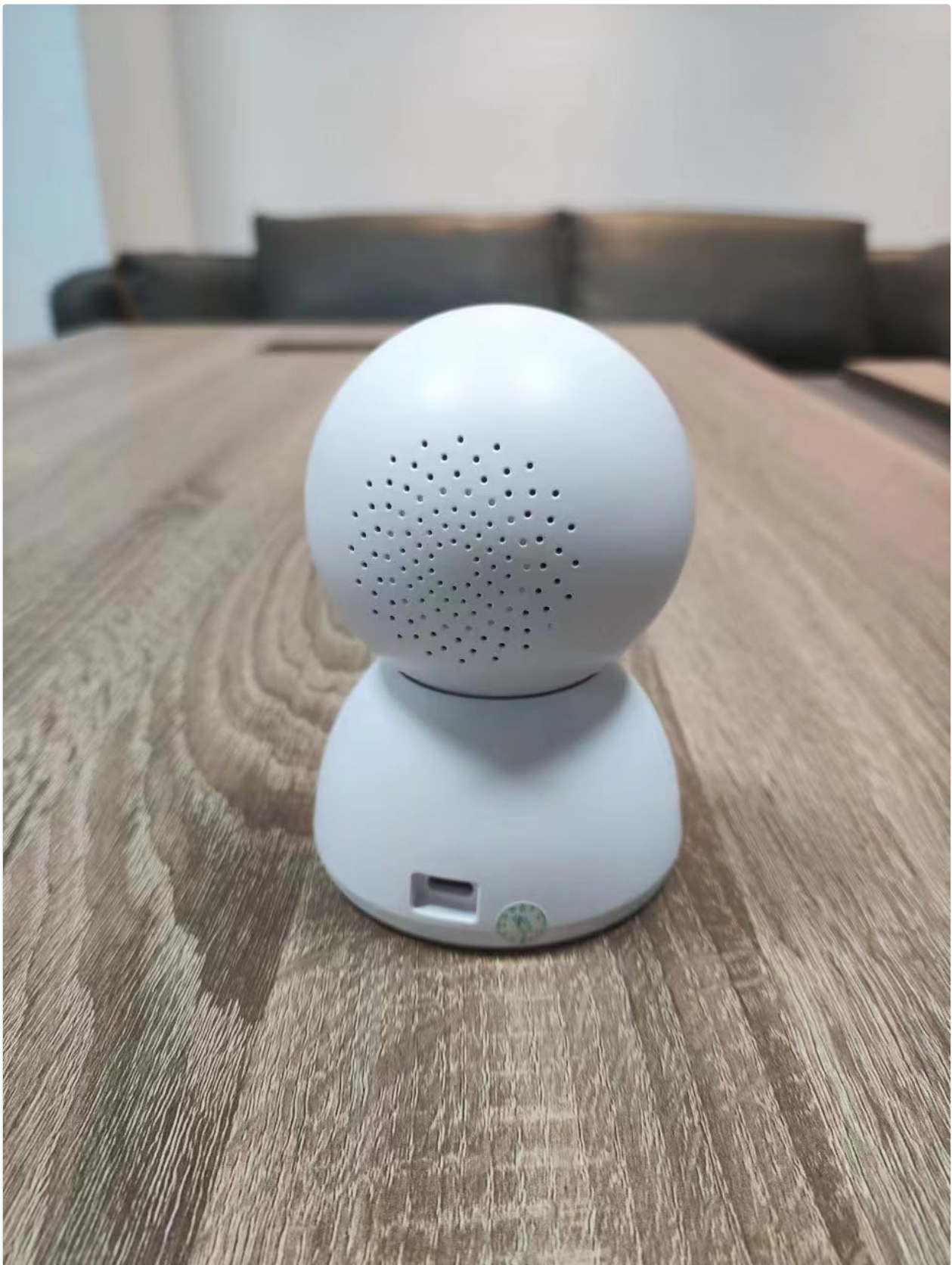
Figure 2: Rear view of the camera, highlighting the speaker grille and USB-C power input.
