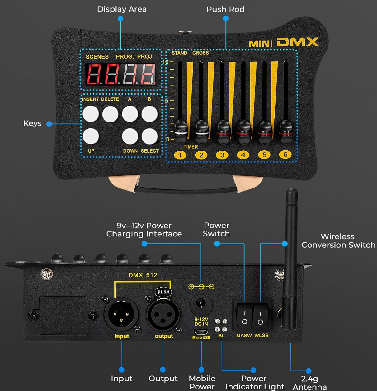
Figure 3.1: Front panel of the DMX controller, highlighting the digital display, six channel faders (push rods), and control buttons for scenes, programs, and navigation.
