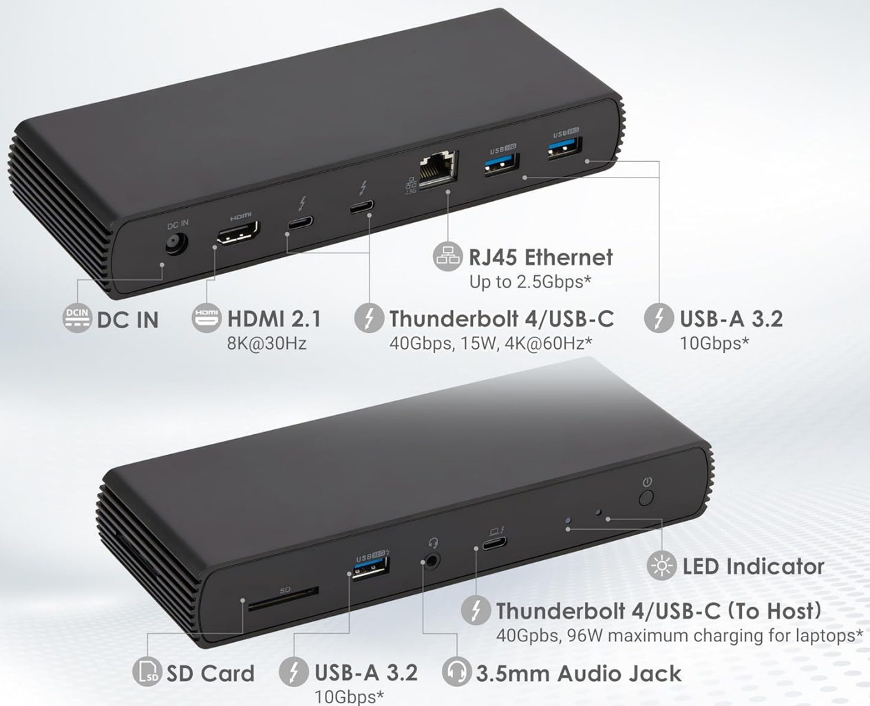
Figure 4.1: Front and Rear View of the Docking Station with Port Labels. This image highlights the various input and output ports available on the docking station, including Thunderbolt 4, USB-A, HDMI, Ethernet, and the SD card slot.
