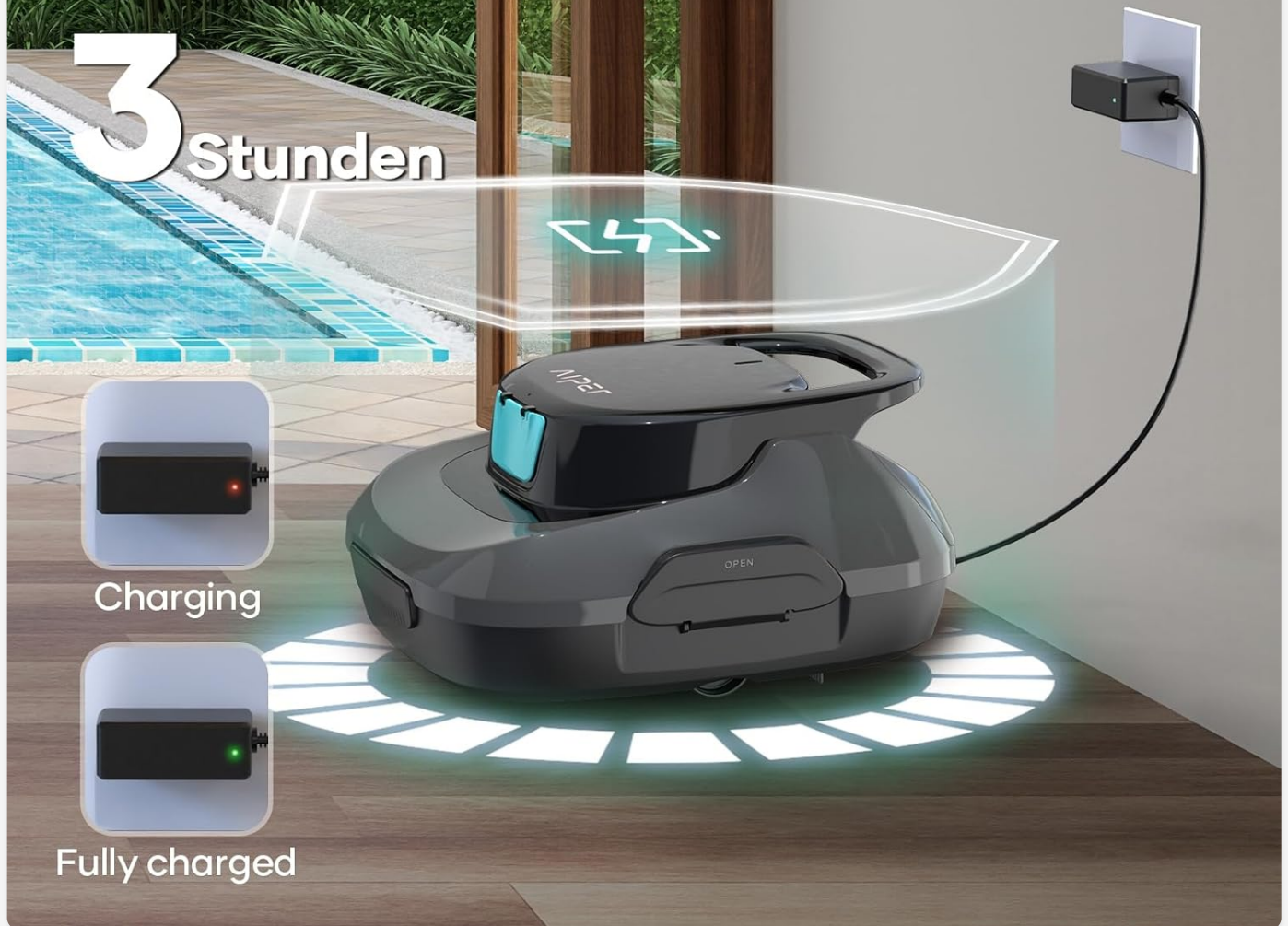
Figure 2: Connect the charger to the device and a power outlet. The LED indicates charging status.
