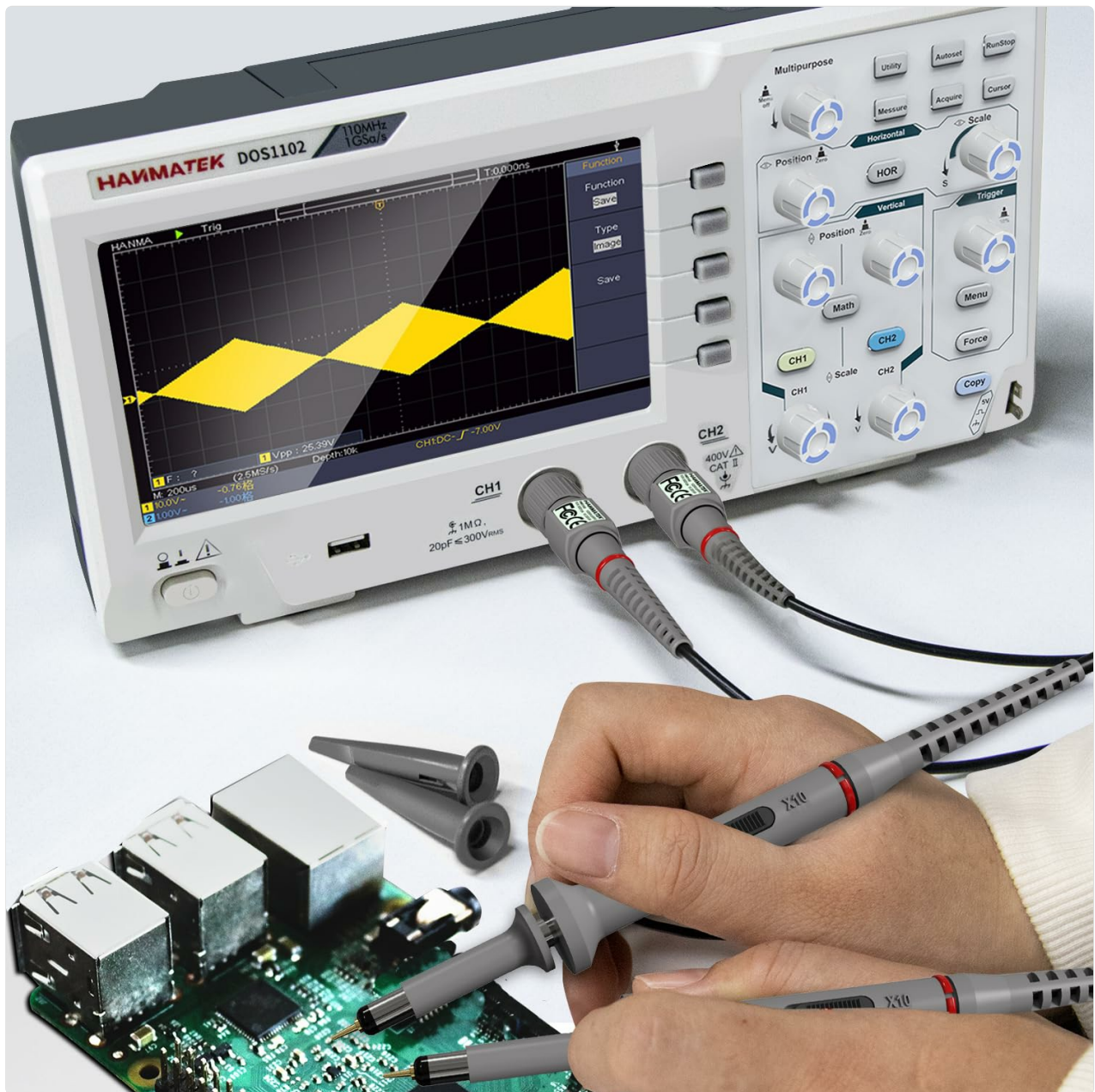
Figure 5.1: Using the HM5100 probe with a desktop oscilloscope.
