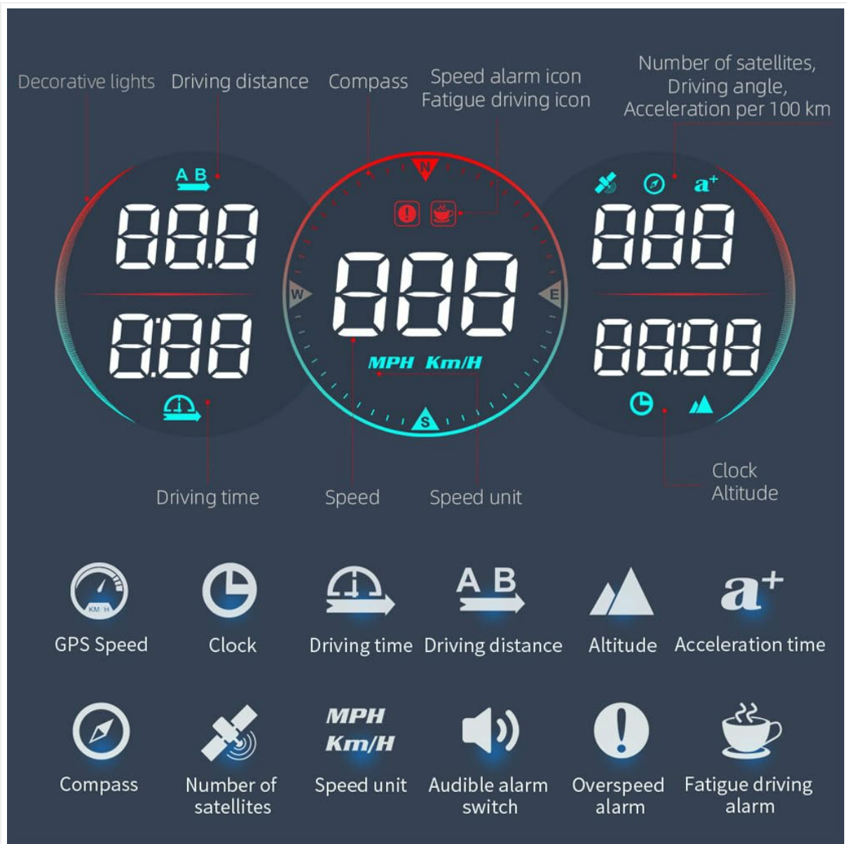
Figure 2: Breakdown of the G17's display elements, including GPS speed, clock, driving time, driving distance, altitude, acceleration time, compass, number of satellites, speed unit, audible alarm switch, overspeed alarm, and fatigue driving alarm.
