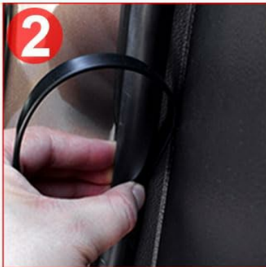
2 Insert the wires into the A-pillar seal
