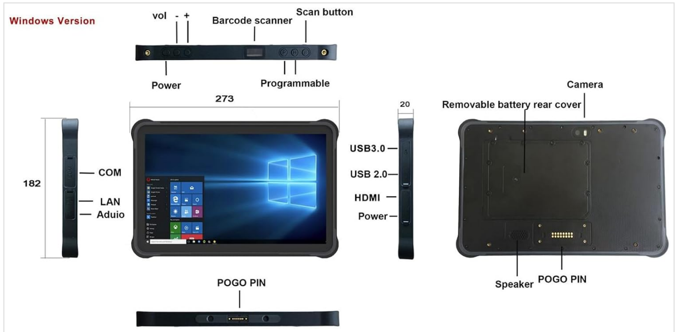
Figure 2: Diagram illustrating the dimensions, ports, and button layout of the Sincoole Rugged Tablet ST11. Key features include volume controls, barcode scanner button, power button, programmable buttons, USB 3.0 ports, RJ45, RS232, HDMI, and a removable battery rear cover.
