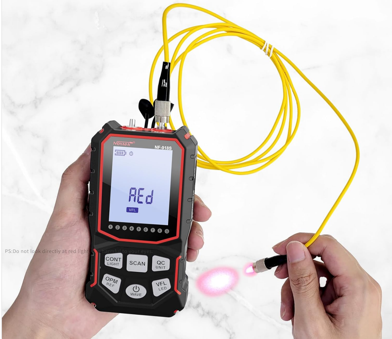
Figure 6.4: Visual Fault Locator. This image shows the NF-918S main unit with its Visual Fault Locator (VFL) function active, emitting a strong red light into a fiber optic cable to help identify breaks or bends.
