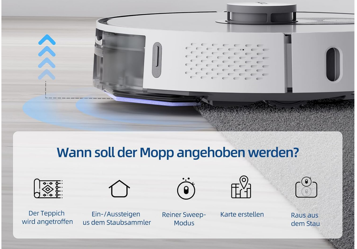
Figure 4.3: Automatic mop lifting mechanism to protect carpets.
