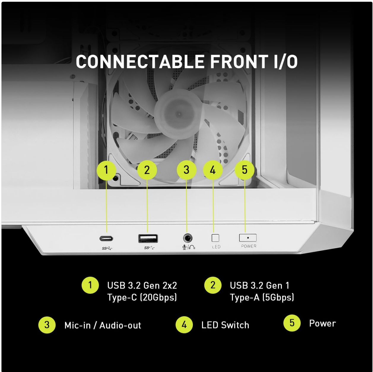
Figure 8: Front I/O panel details.
