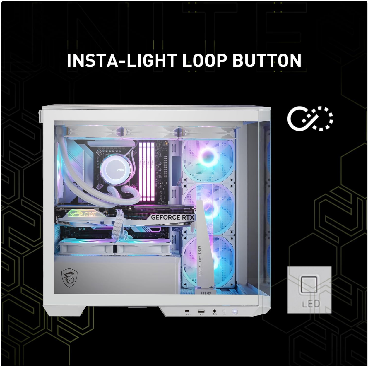
Figure 3: Internal cooling system with ARGB fans.
