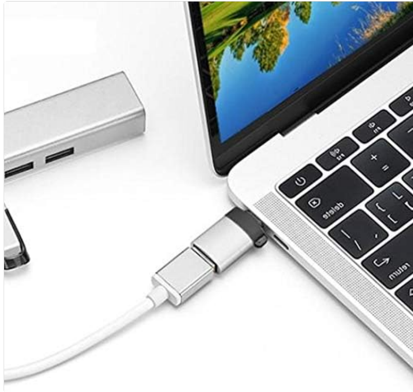
Image 3.1: The PortChanger adapter connected to a laptop's USB-C port, then to a USB hub, demonstrating its role in expanding connectivity.
