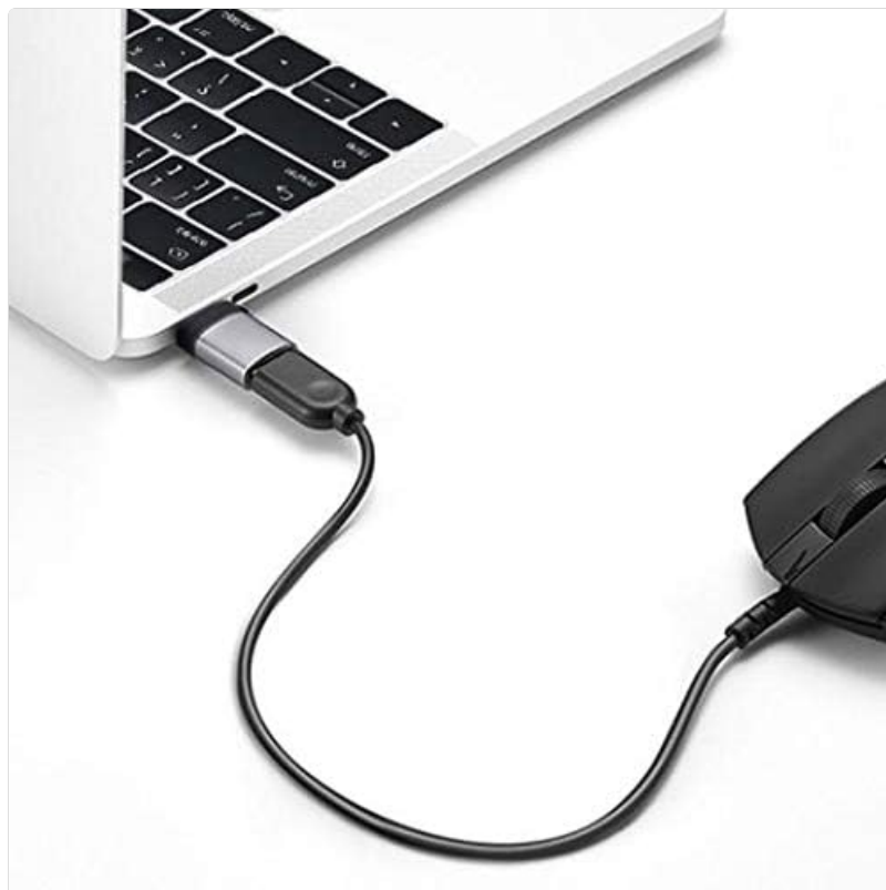
Image 4.2: The PortChanger adapter facilitating the connection of a USB mouse to a laptop's USB-C port.
