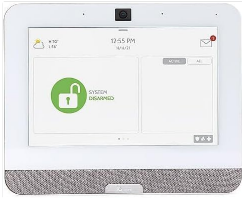
Figure 5.2: The IQ Panel 4 display when the system is disarmed, indicated by a green unlocked padlock icon and corresponding text.
