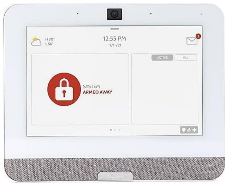
Figure 5.1: The IQ Panel 4 display when the system is armed in 'Away' mode, indicated by a red padlock icon and corresponding text.
