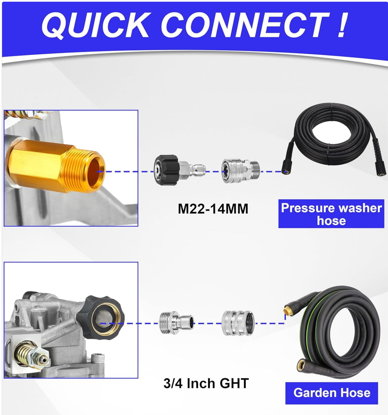
Figure 4: Quick-connect fittings for easy hose attachment.
