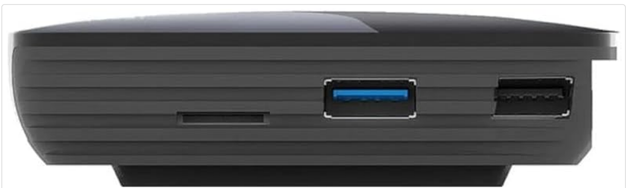
Figure 3.2: Side view of the Vontar X3 Android TV Box, displaying additional connectivity options such as USB ports (one
