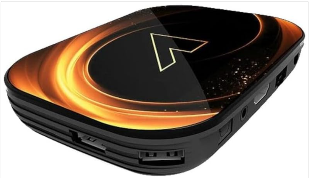
Figure 3.1: Rear view of the Vontar X3 Android TV Box, showing various ports including HDMI, Ethernet (LAN), and DC power input. These ports are essential for connecting the device to a television and power source.
