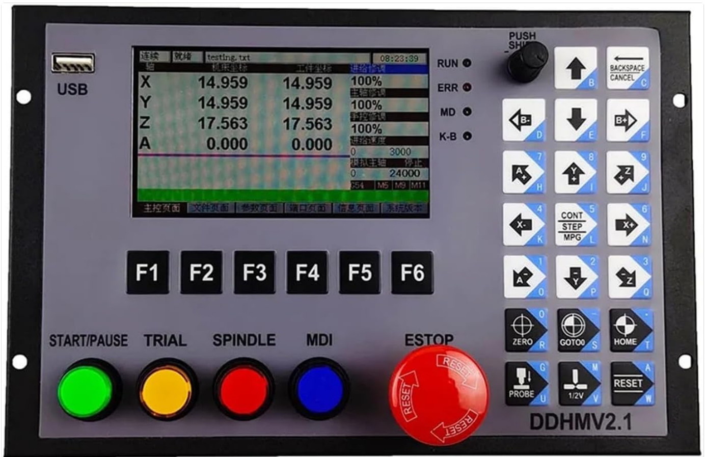
Figure 4.2: Front panel of the DDHVM2.1 controller, featuring the display, function keys (F1-F6), operational buttons (START/PAUSE, SPINDLE, MDI, ESTOP), and navigation controls.
