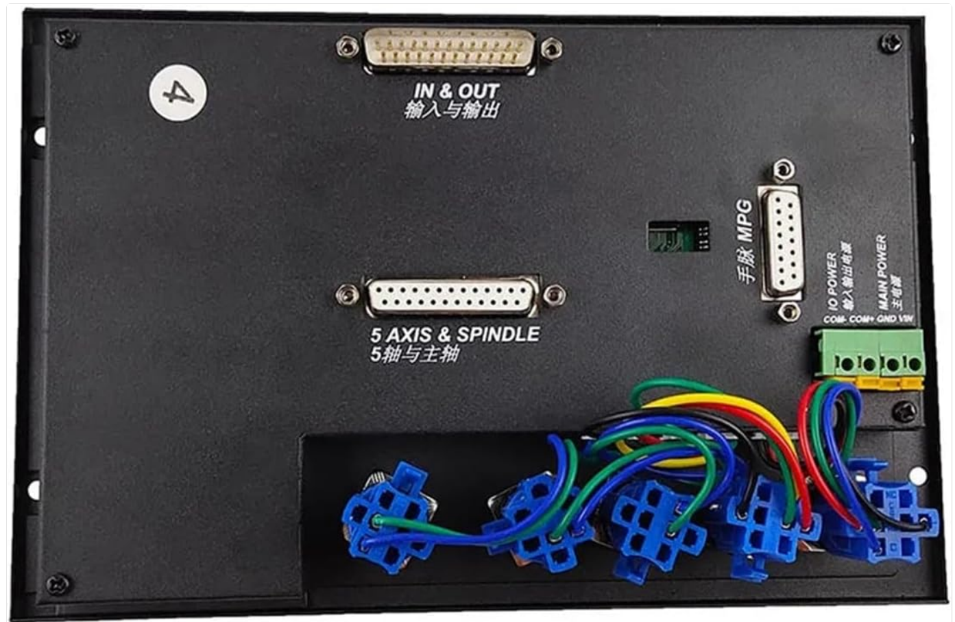
Figure 4.1: Rear panel of the DDHVM2.1 controller, illustrating the IN & OUT, 5 AXIS & SPINDLE, MPG, IO POWER, and MAIN POWER ports.
