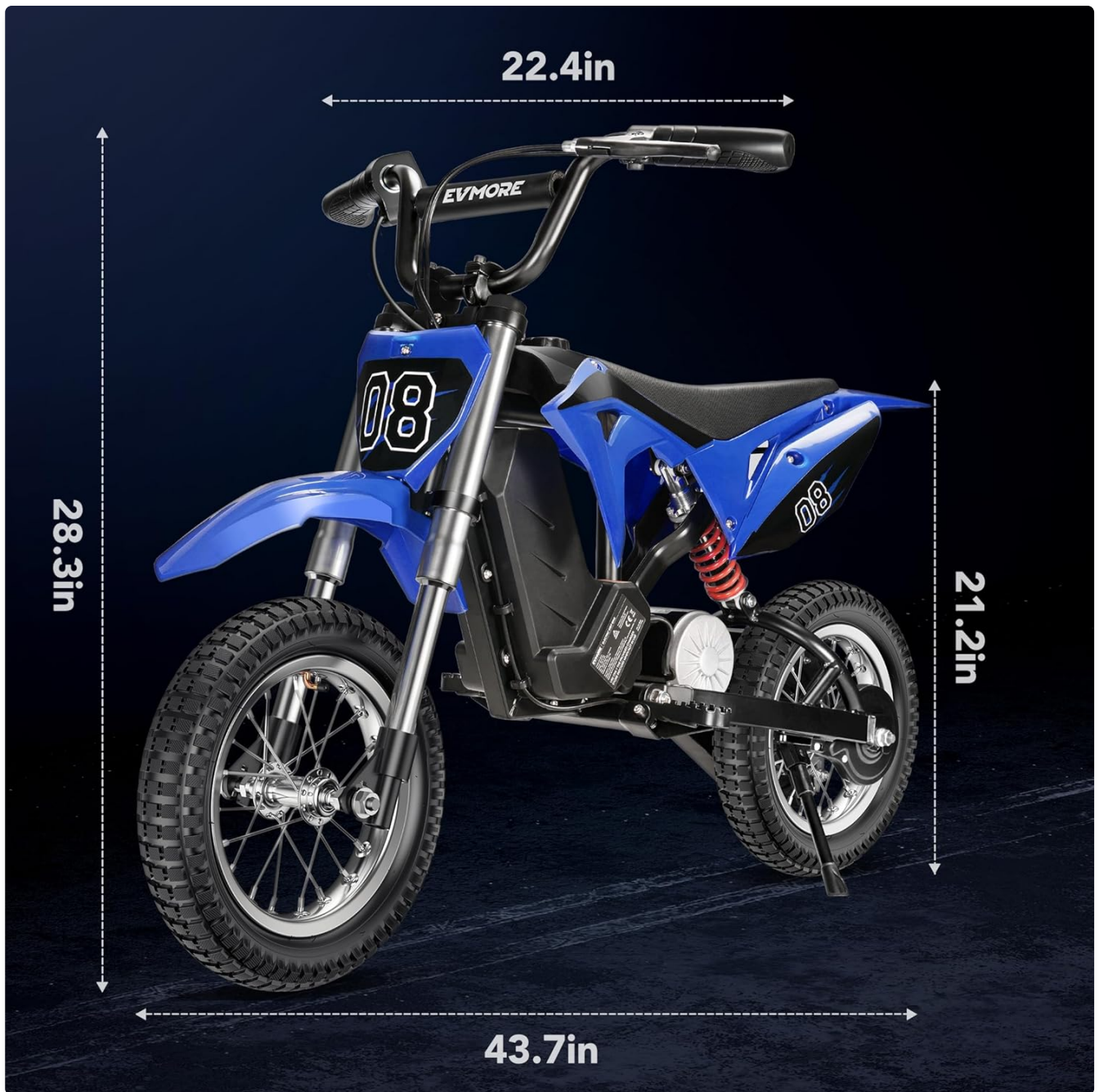
Figure 7: Product Dimensions. This diagram provides key measurements of the electric motorcycle, including its length (43.7 inches), handlebar width (22.4 inches), and height (28.3 inches), offering a clear visual reference for its size.
