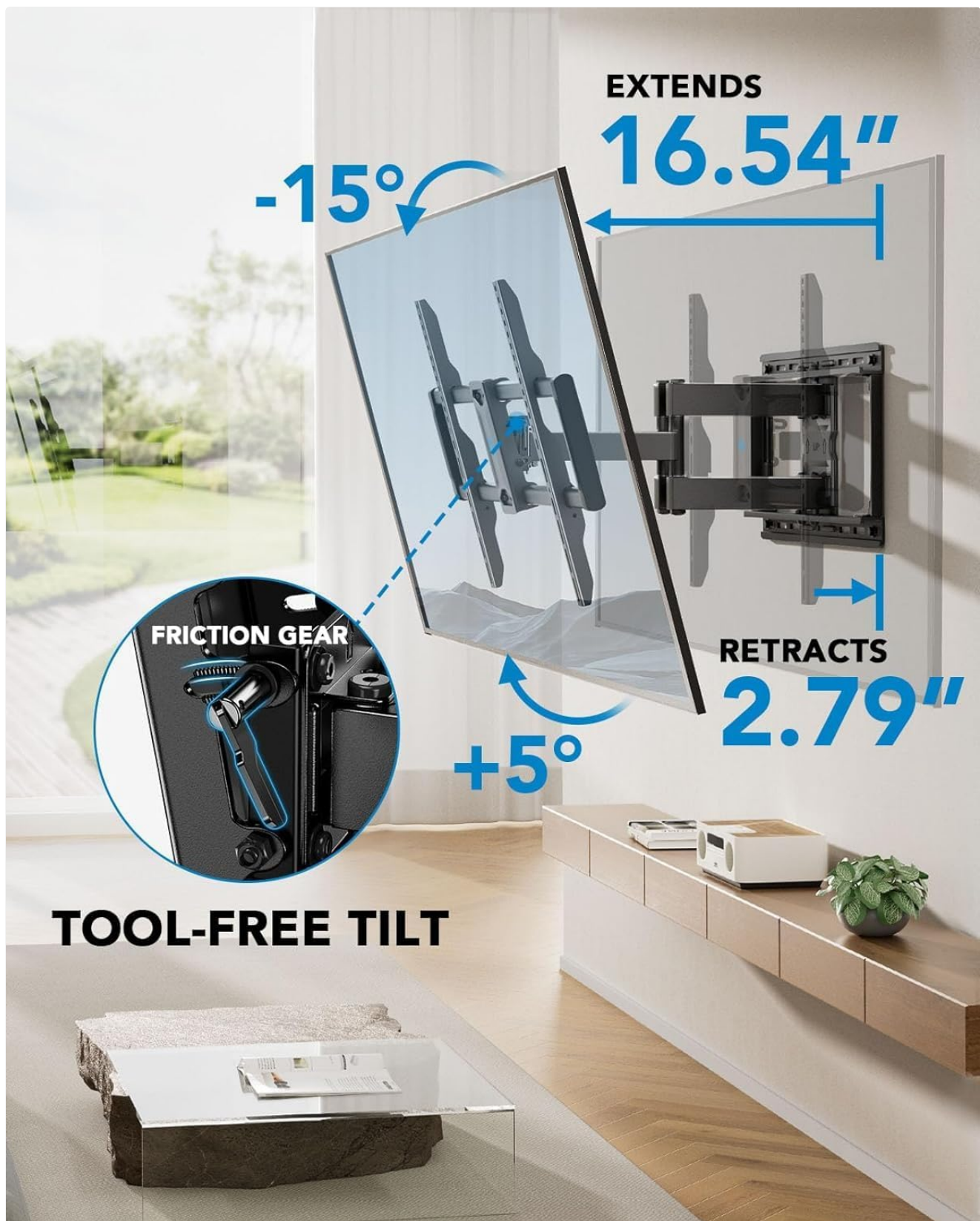
Figure 3: Demonstrates the mount's extension from 2.79 inches to 16.54 inches and tool-free tilt range of +5° to -15°.
