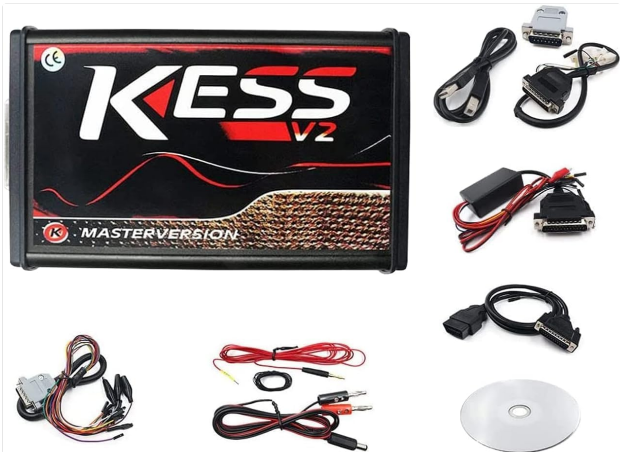
Figure 2.1: The QKVCX Kess V5.017 main unit along with its complete set of accessories, including various connection cables, adapters, and the software CD.
