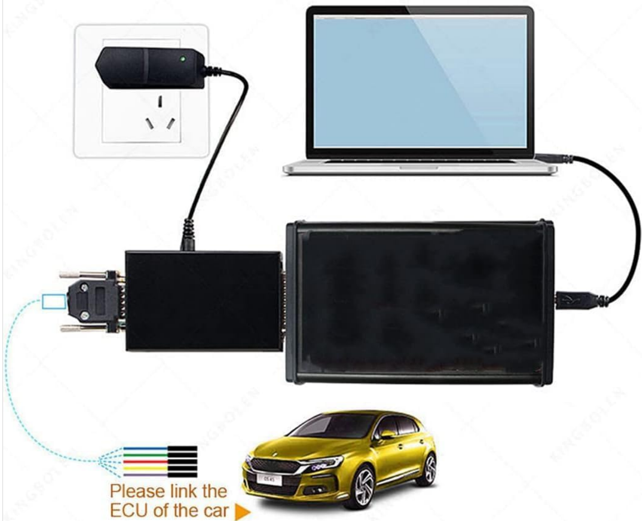
Figure 5.1: This diagram demonstrates how to connect the Kess V5.017 to a vehicle's OBD2 port for ECU programming, with the device linked to a laptop.
