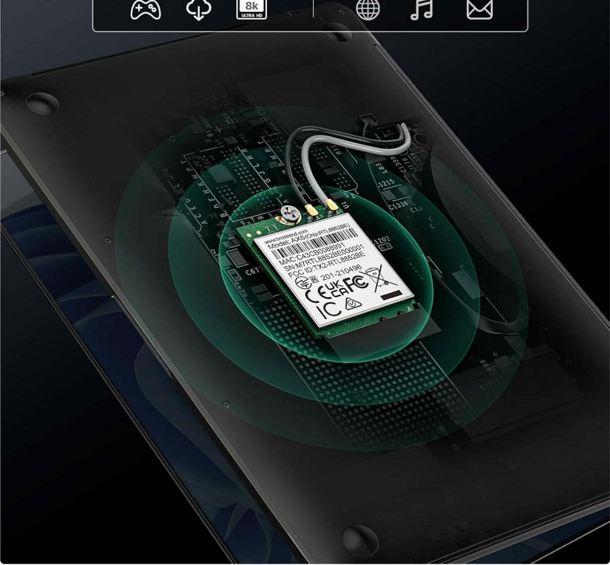
Image: The BrosTrend AX1800 M.2 WiFi 6 card shown installed within a laptop, illustrating its compact size and placement.
