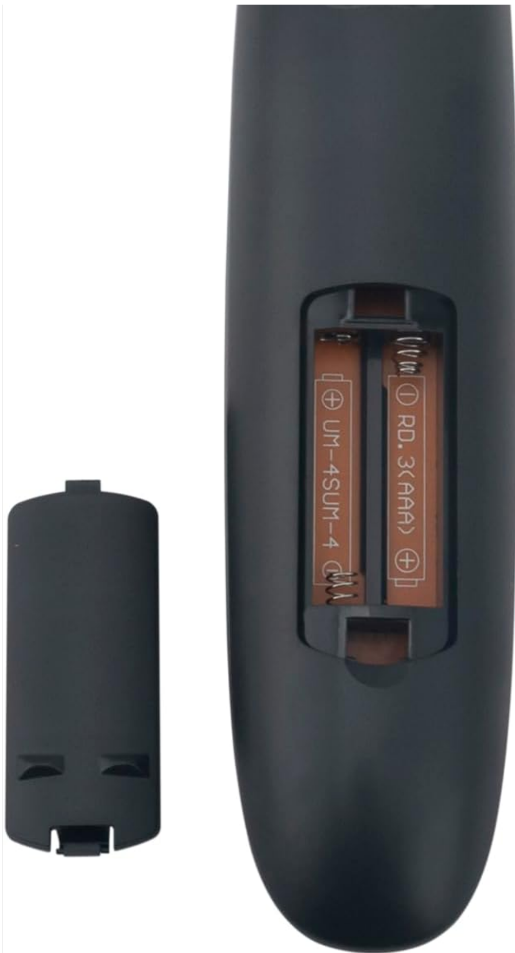
Figure 2.1: Battery compartment with cover removed, showing battery orientation.
