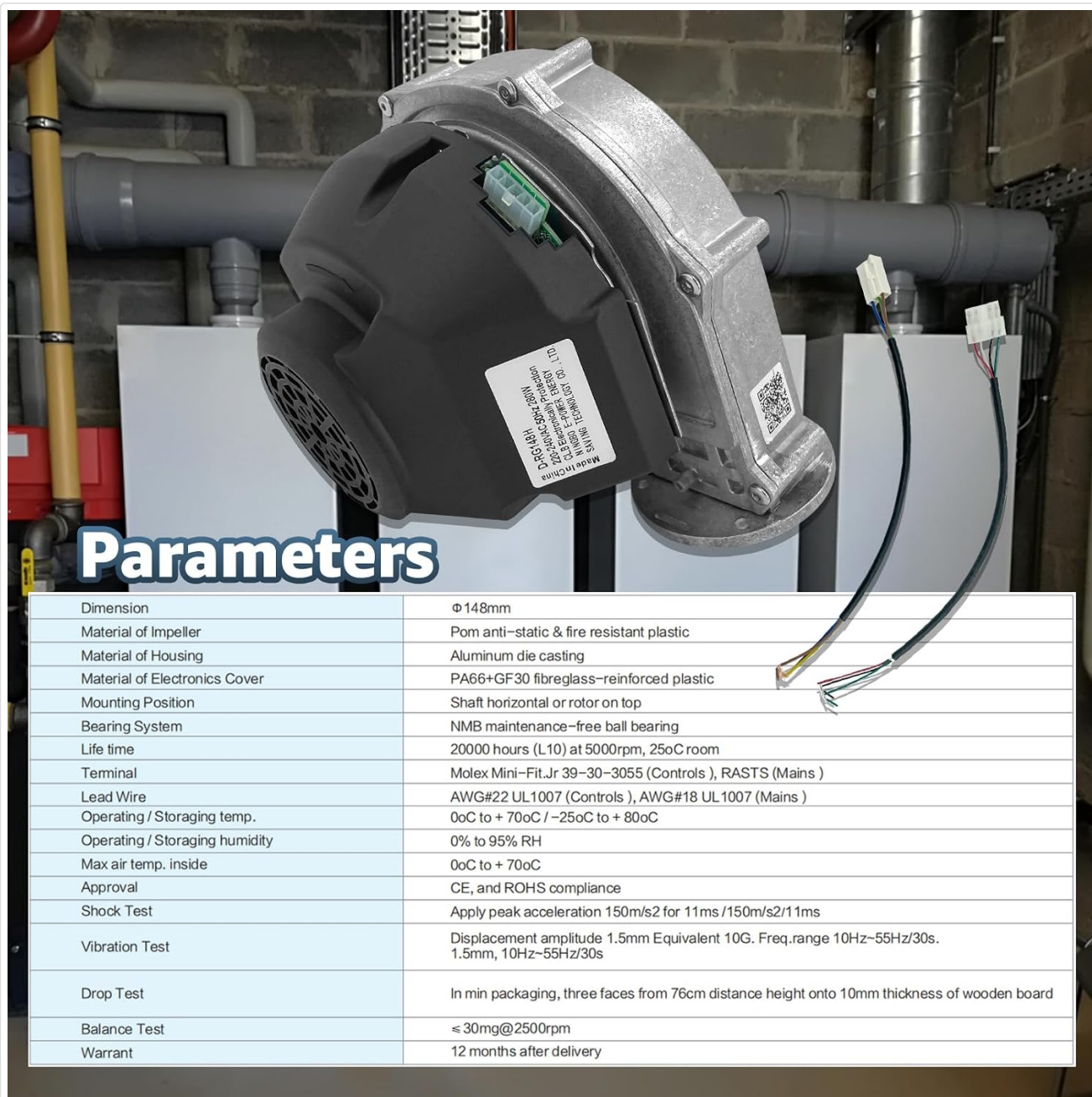
Figure 4.2: Detailed physical parameters and environmental ratings of the blower cooling fan.
