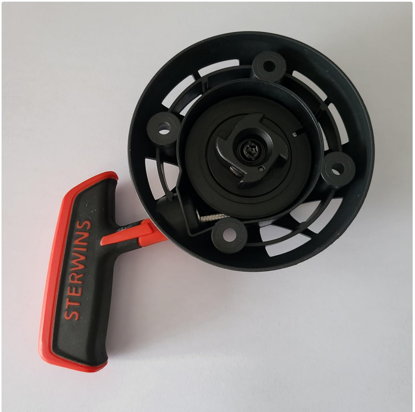
Figure 2: Rear view of the starter assembly, illustrating the internal winding mechanism and the four mounting holes.
