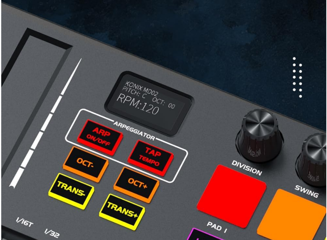
Figure 5: OLED screen displaying PITCH, OCTAVE, and tempo, with ARP and TAP TEMPO buttons.
