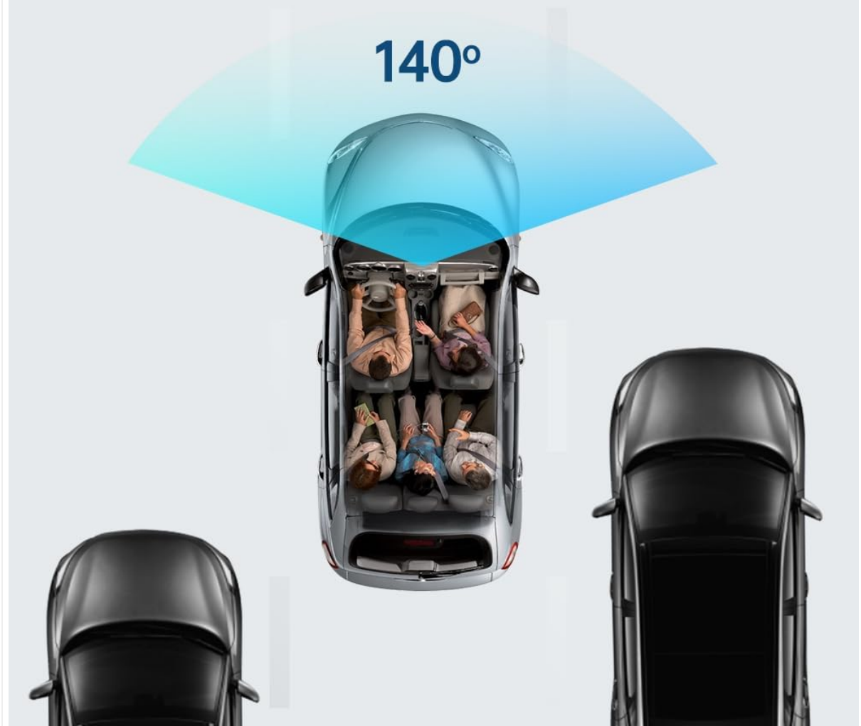
Figure 2: Illustration of the 140-degree wide-angle view provided by the dash cam.
