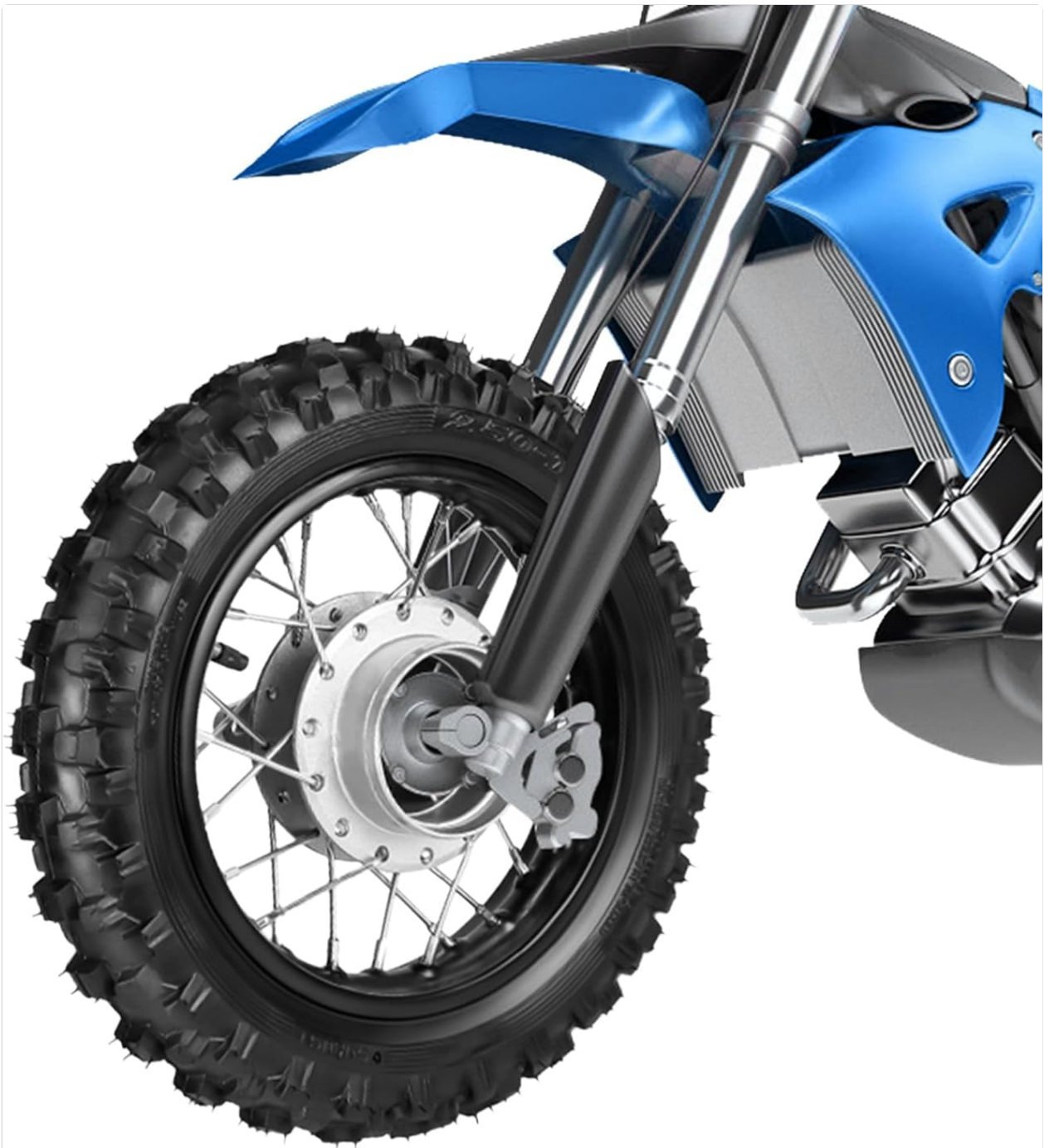
Figure 3: Example of a wheel assembly installed on a dirt bike.
