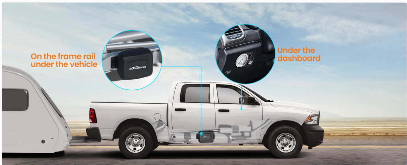
Image: Recommended mounting locations for the compressor and gauge.
