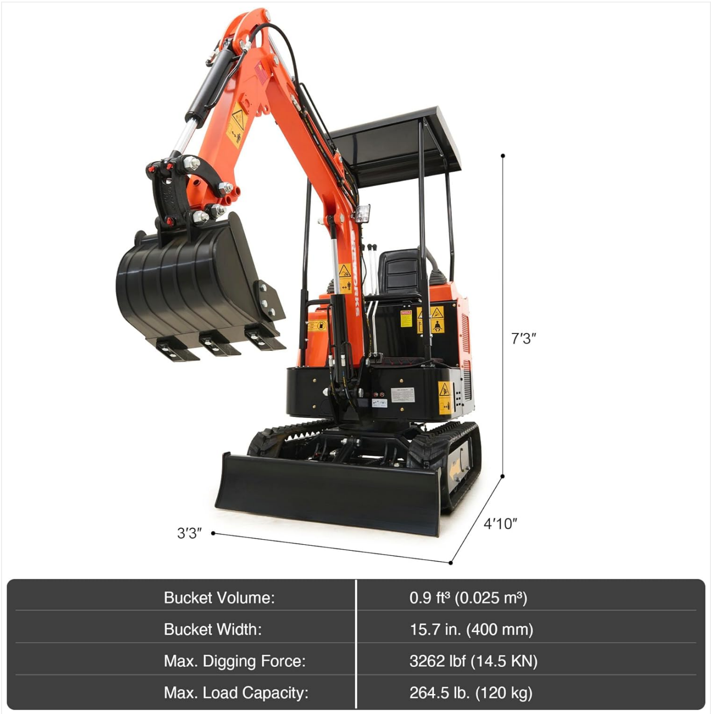
Figure 3.2: Visual representation of the mini excavator's key dimensions and performance specifications.
