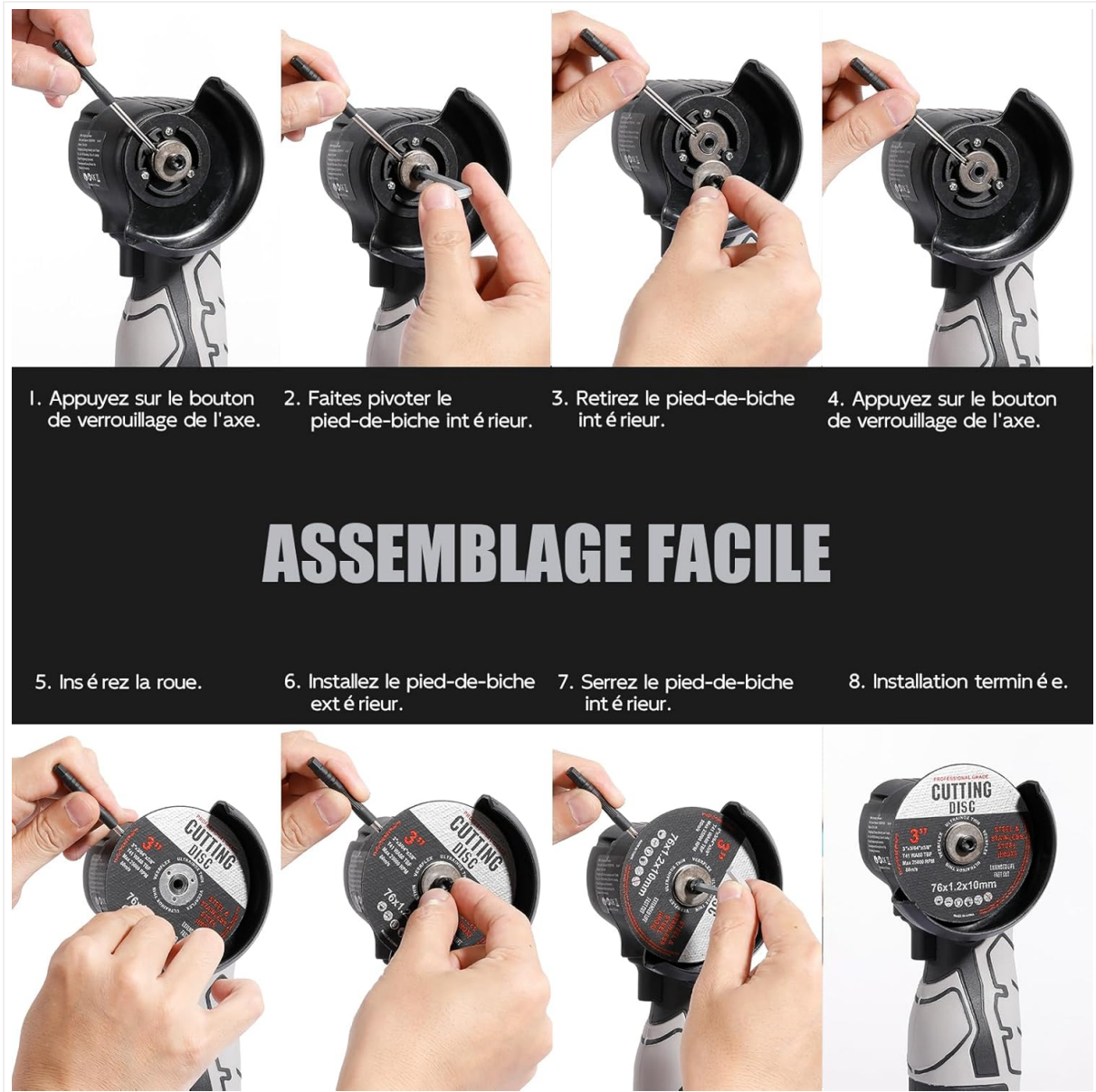
Figure 5.1: Easy assembly steps for installing a cutting disc.
