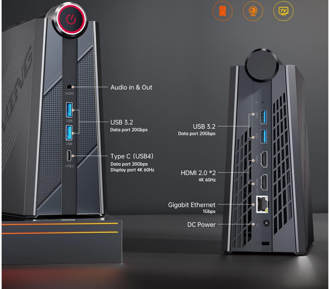
Figure 3.4: Overview of the various ports available on the KAMRUI AM08PRO, including USB, HDMI, Type-C, and Ethernet.
