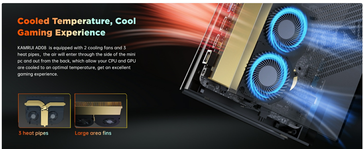
Figure 3.6: Diagram illustrating the internal cooling components, including dual fans and heat pipes, designed for efficient heat dissipation.
